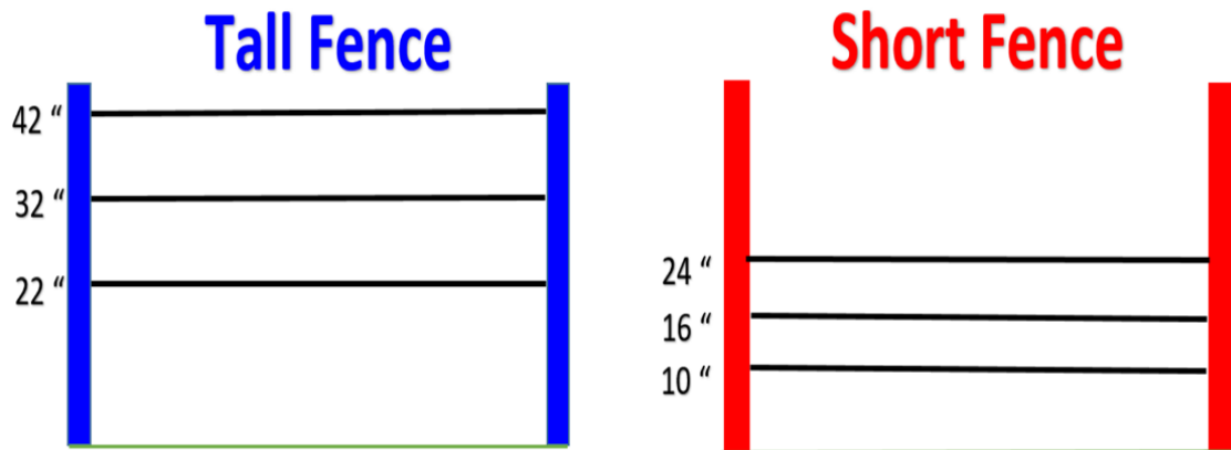
Figure 5. Two fence designs used in the study. The tall fence design was modeled after the NRCS specifications for a wildlife friendly boundary fence in Montana (House Bill No. 557, Montana Legislature). The short fence design was modeled after a 3 wire electric fence that proved effective at deterring black bears in Michigan (Otto 2013).
