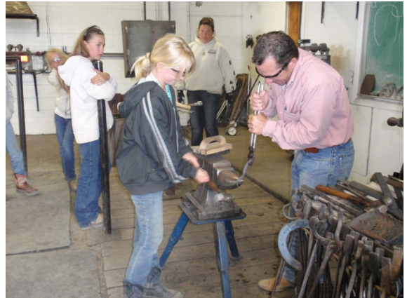
Schuyler German, of Belgrade, MT, builds a hoof pick from a horseshoe with the help of Shannon Moreaux.
