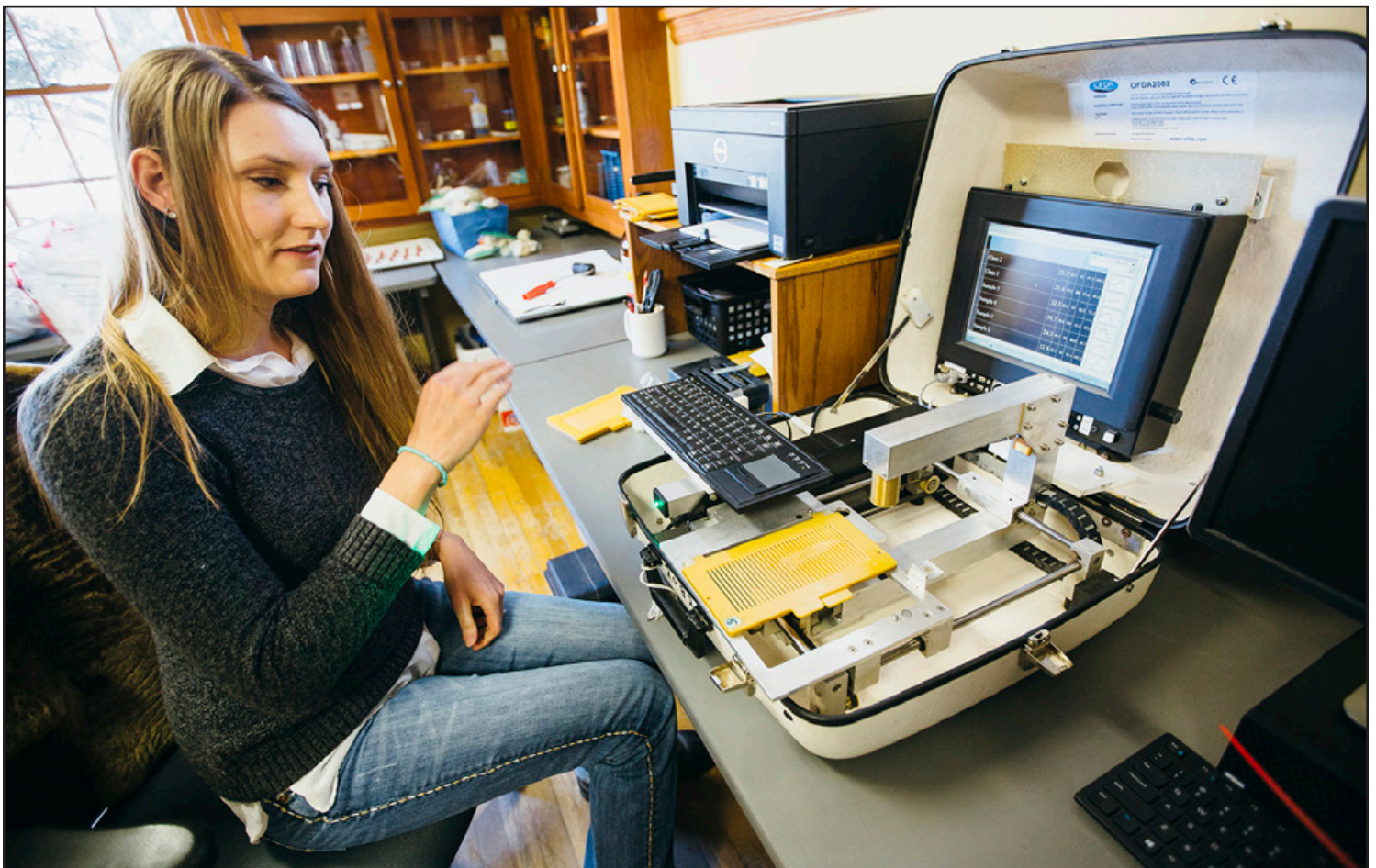
Devon demonstrates use of a portable wool fiber analyzer at the Wool Lab on the campus of Montana State University
